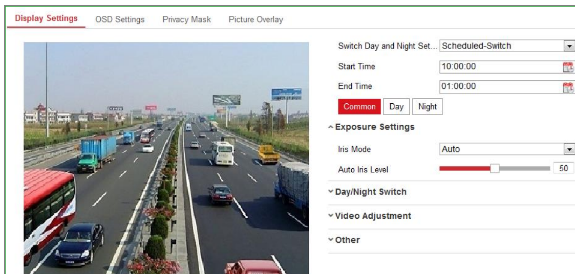
Figure 9-5 Day/Night Scheduled-Switch Configuration Interface
