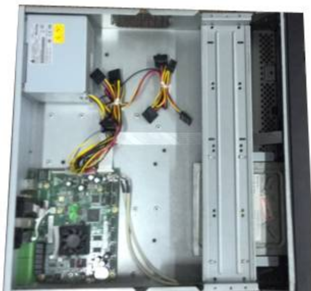
Figure 3-45 Put bracket back
