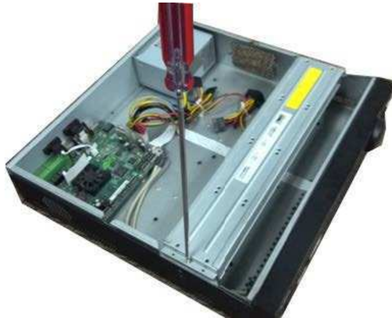
Figure 3-37 Open the top cover
