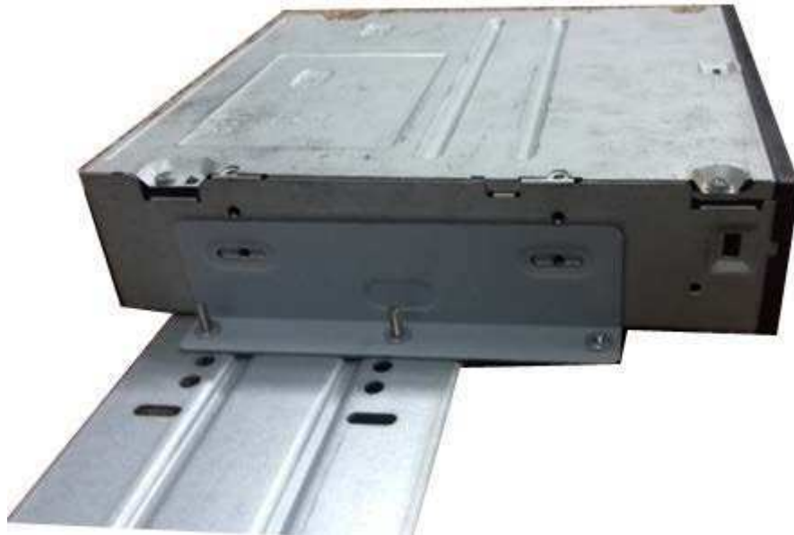
Figure 3-43 Install SATA burner
