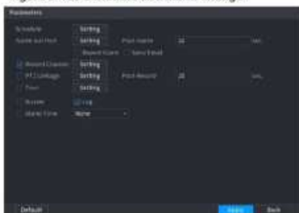
Figure 5-163 Schedule and alarm linkage
