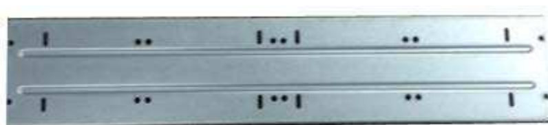
Figure 3-38 Take out HDD bracket
