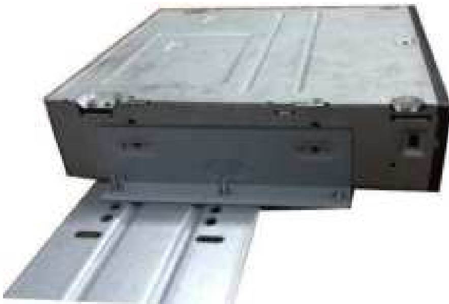
Figure 3-43 Install SATA burner
