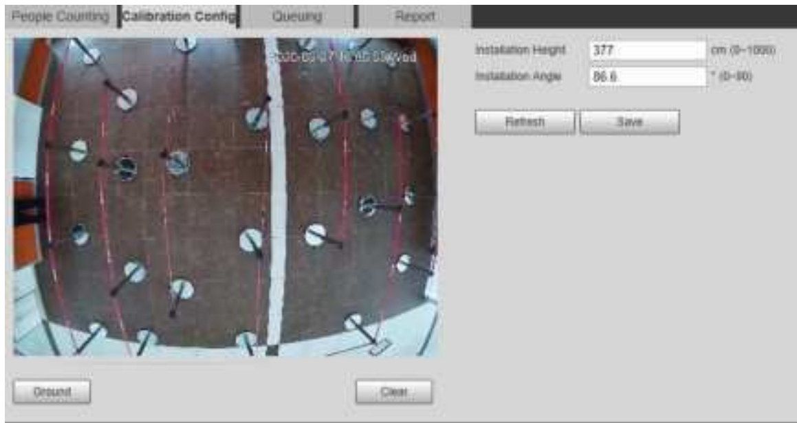
Figure 5-67 Calibration configuration (stereo analysis)
