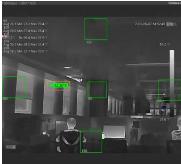
Figure 4-7 Real-time spot temperature monitoring
