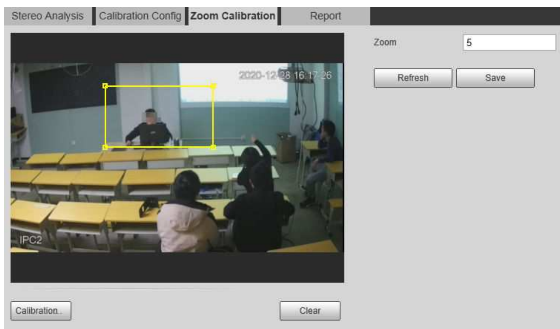
Figure 5-81 Calibration configuration (stereo analysis)
