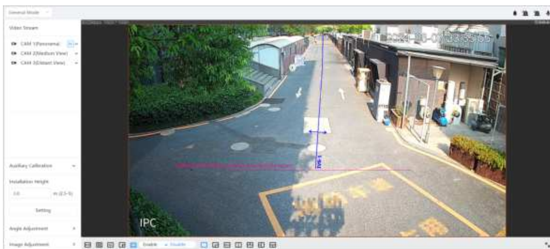
Figure 7-7 Configure auxiliary calibration
