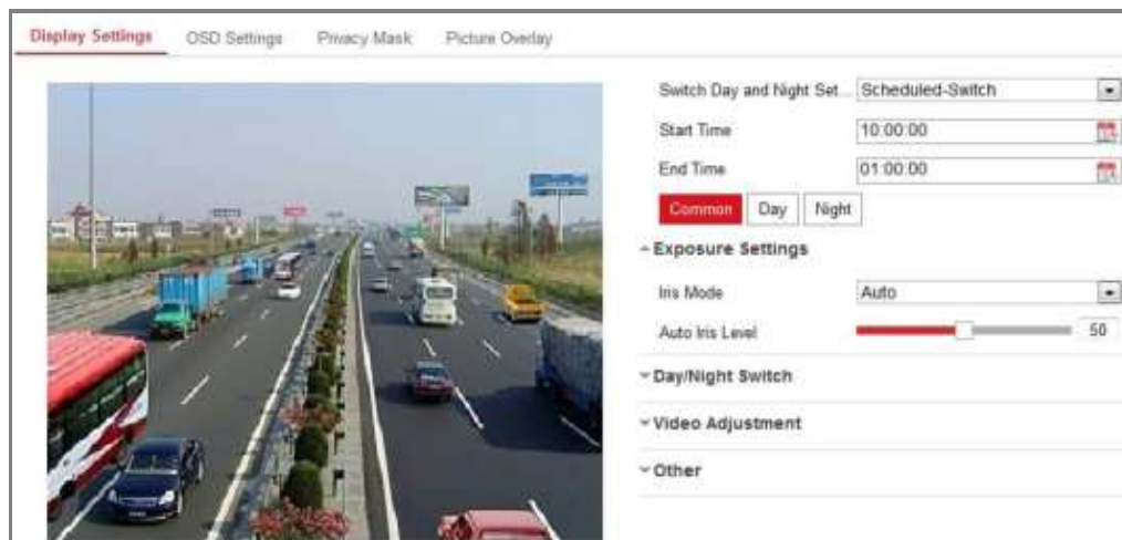
Figure 9-5 Day/Night Scheduled-Switch Configuration Interface
