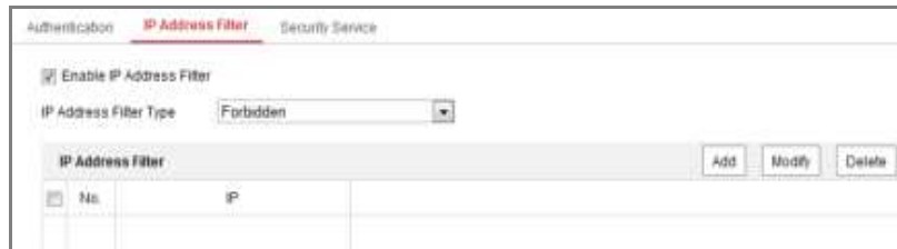
Figure 6-17 IP Address Filter Interface
