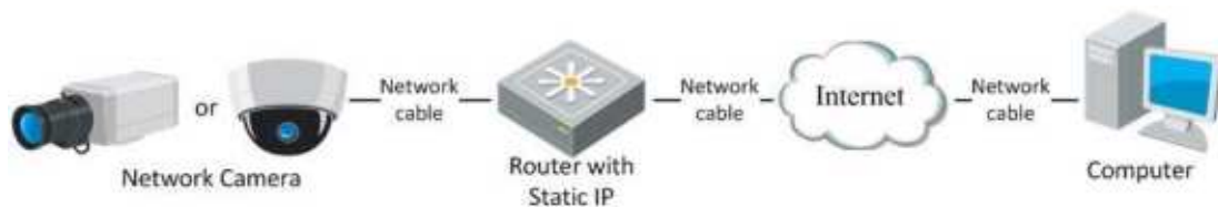
Figure 2-6 Accessing the Camera through Router with Static IP
