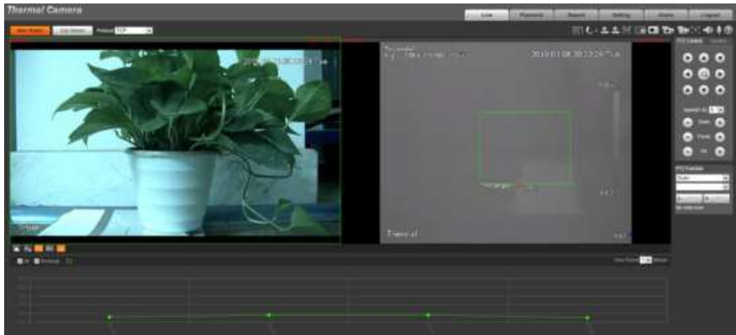
Figure 3-6 Temperature recording area
