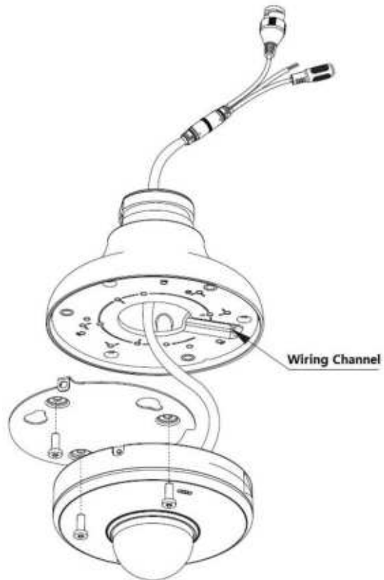
Figure 4-4 Installing the mounting plate
