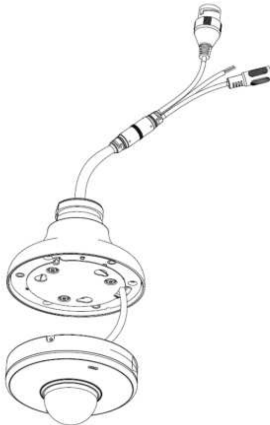
Figure 4-5 Hanging the speed dome
