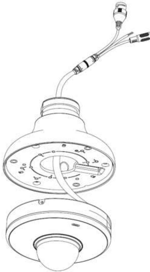
Figure 4-3 Pulling the speed dome cables
