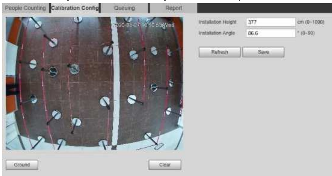
Figure 5-67 Calibration configuration (stereo analysis)
