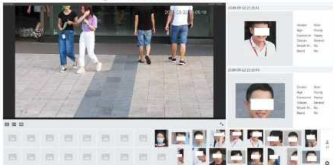
Figure 8-20 Face detection result
