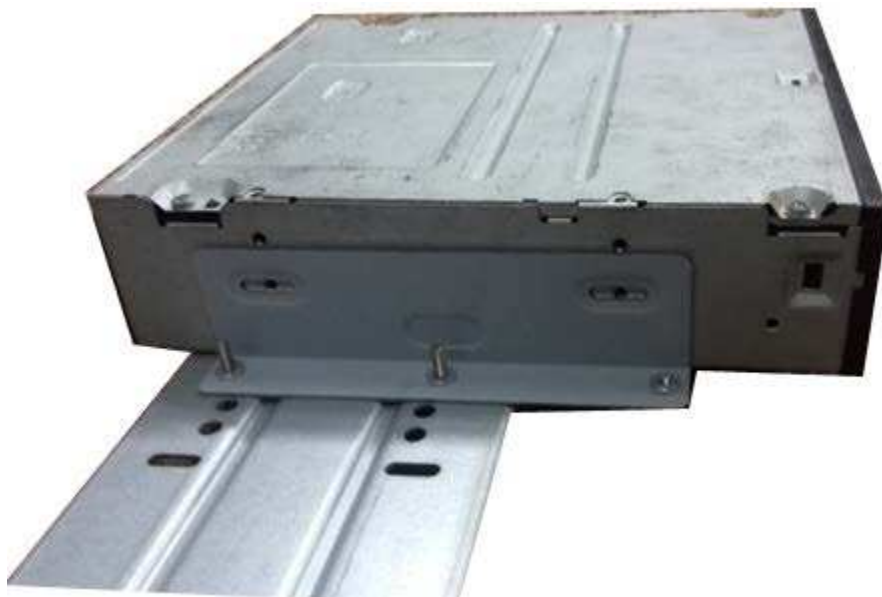
Figure 3-38 Install SATA burner
