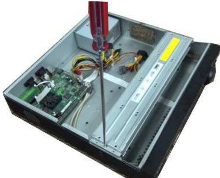
Figure 3-37 Open the top cover
