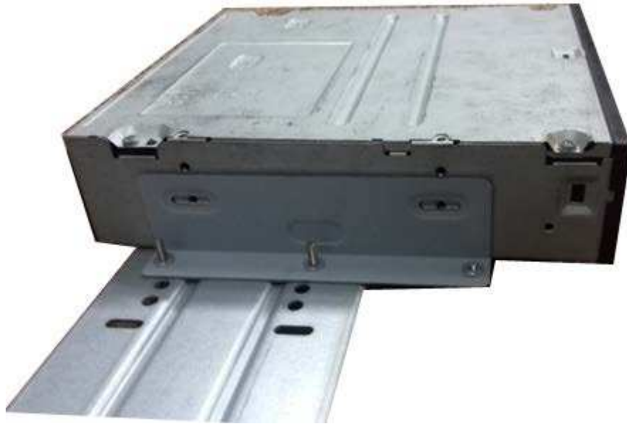
Figure 3-43 Install SATA burner
