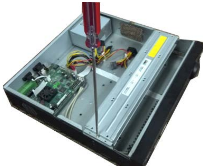
Figure 3-36 Open the top cover
