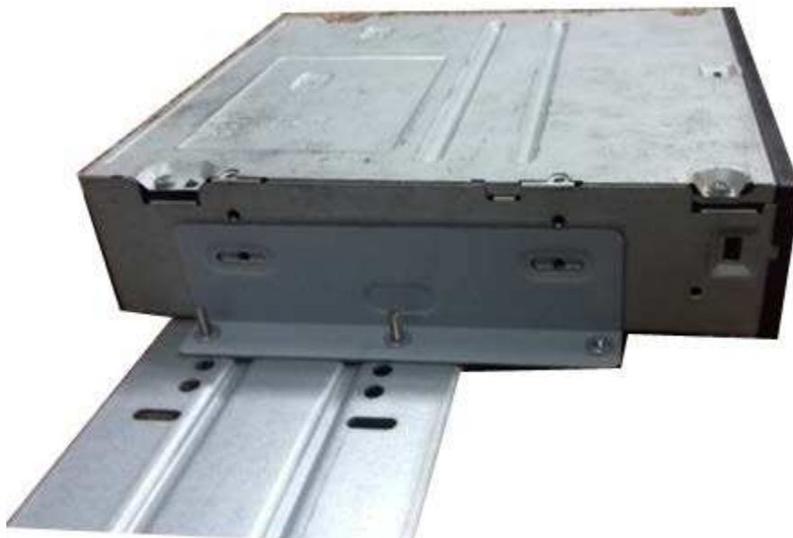
Figure 3-38 Install SATA burner
