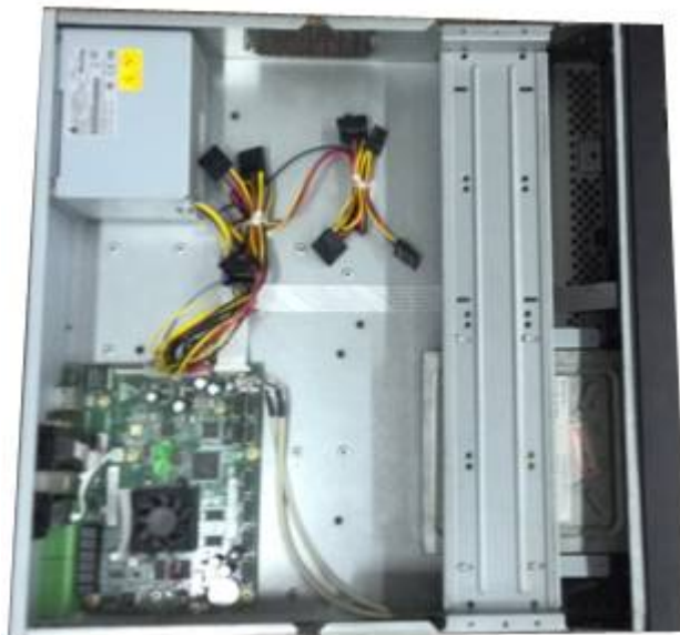
Figure 3-40 Put bracket back
