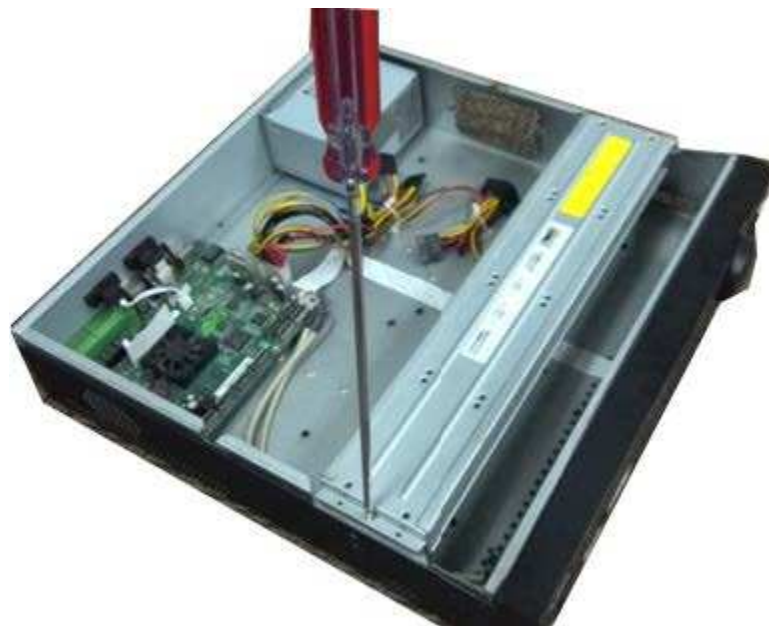
Figure 3-32 Open the top cover
