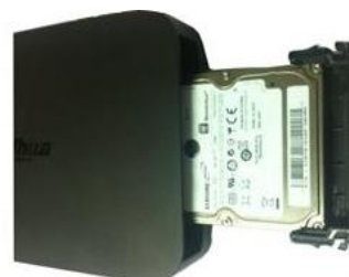
③ Put the HDD into the device
