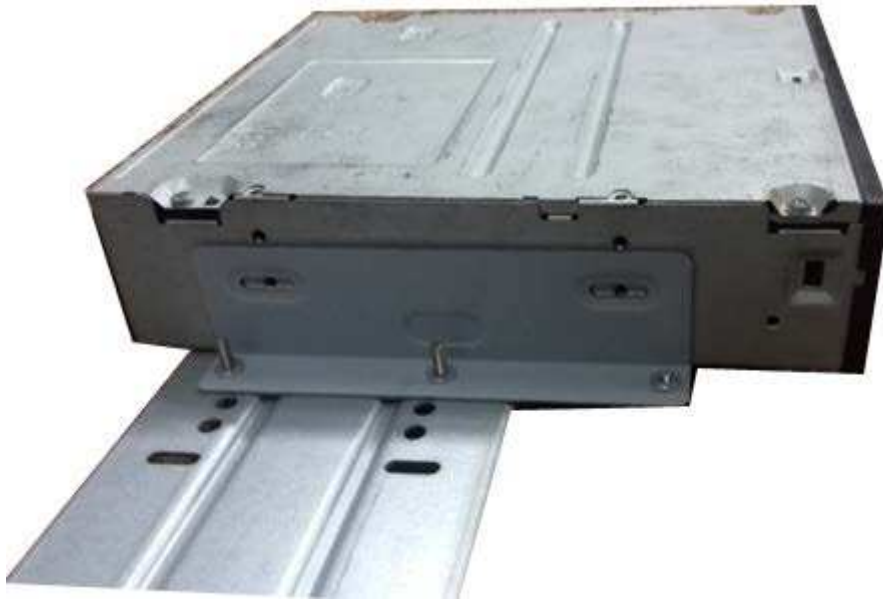
Figure 3-43 Install SATA burner
