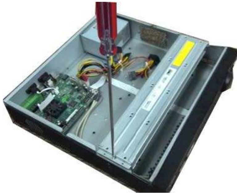
Figure 3-37 Open the top cover
