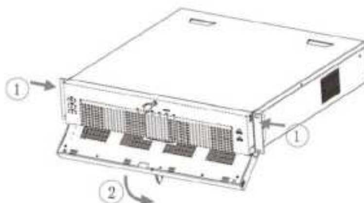
Figure 3-29 Open front panel
