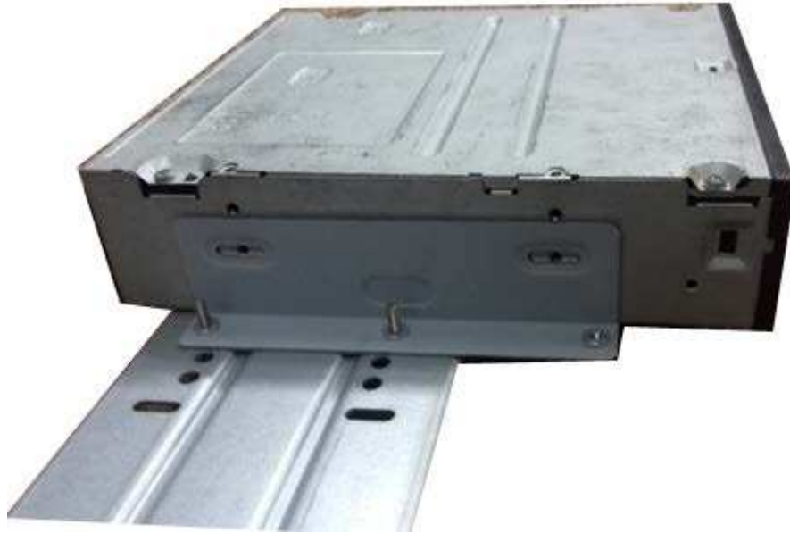
Figure 3-43 Install SATA burner
