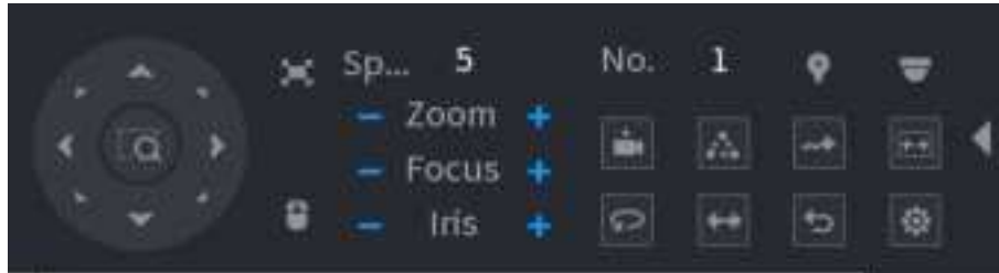
Figure 5-43 Expanded PTZ control panel
