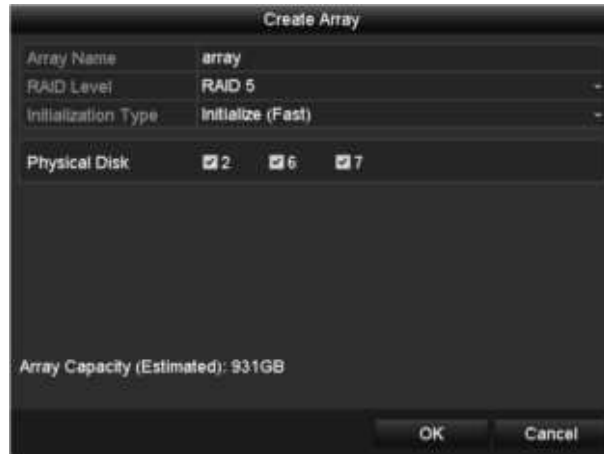
Figure 13. 8 Create Array Interface
