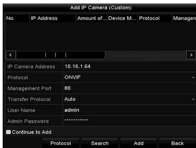
Figure 2.22 Custom Adding IP Camera Interface
