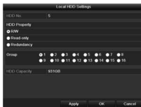
Figure 13. 15 Local HDD Settings Interface
