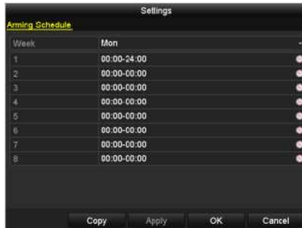
Figure 8. 16 Set Arming Schedule of Alarm Output
