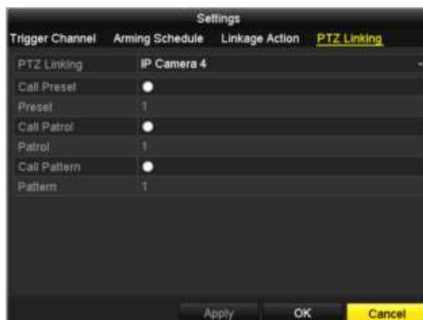
Figure 8. 6 Set PTZ Linking of Alarm Input
