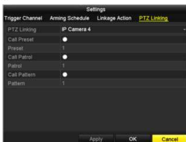
Figure 8. 7 Set PTZ Linking of Alarm Input
