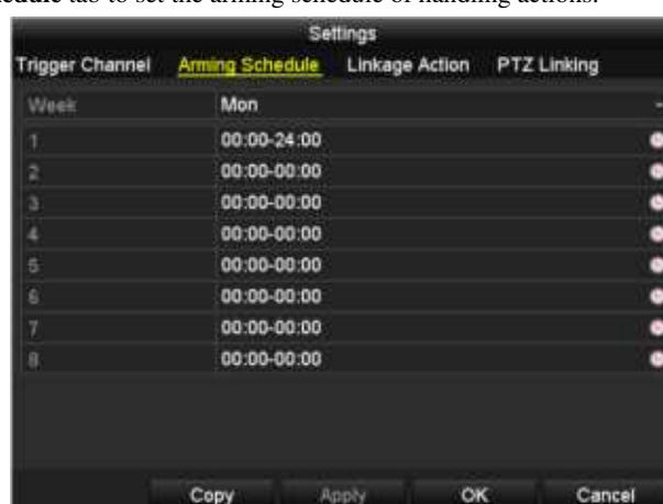
Figure 8.14 Set Arming Schedule of VCA Alarm
