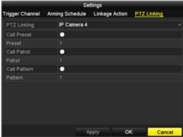
Figure 8. 7 Set PTZ Linking of Alarm Input
