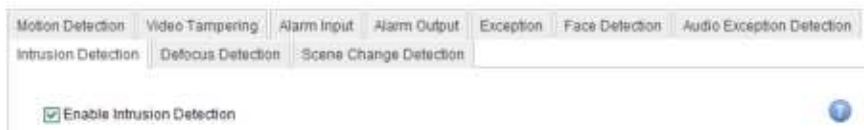
Figure 6. 6 Setting Intrusion Detection on IP Camera
