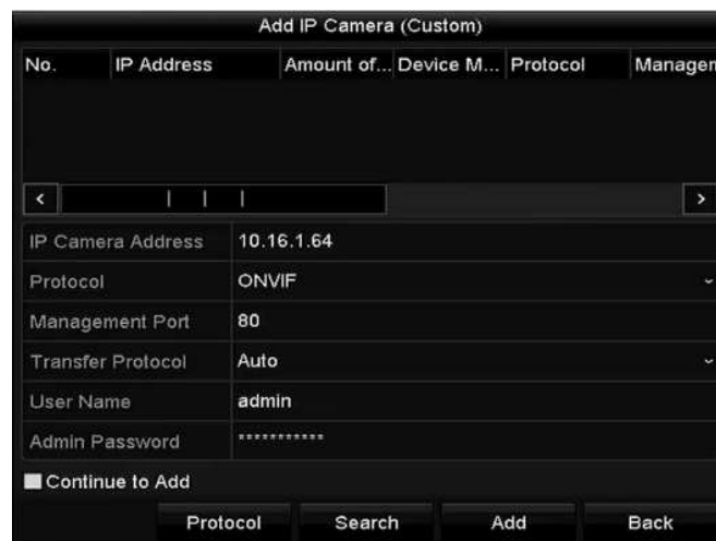
Figure 2. 28 Custom Adding IP Camera Interface
