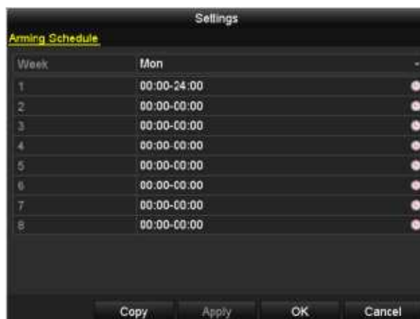
Figure 8. 17 Set Arming Schedule of Alarm Output
