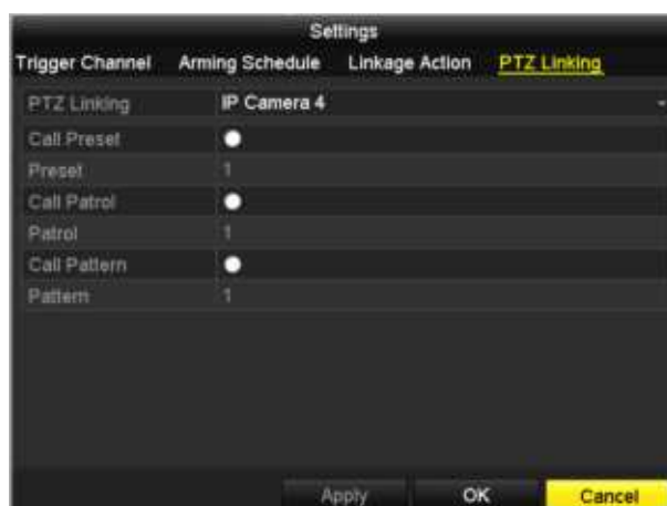
Figure 8. 7 Set PTZ Linking of Alarm Input
