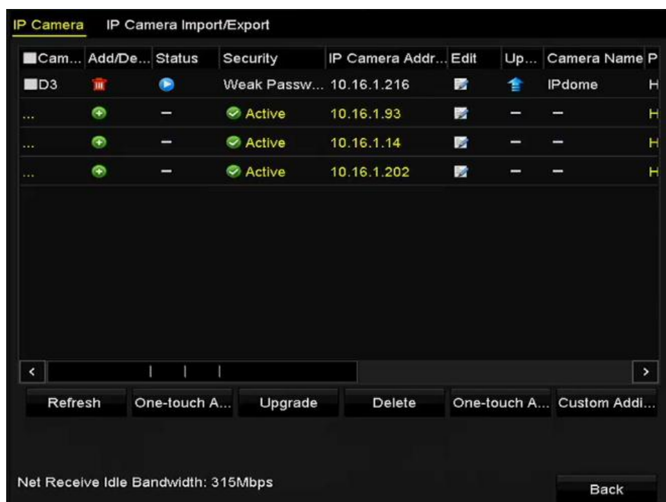
Figure 2. 23 Successfully Added IP Cameras
