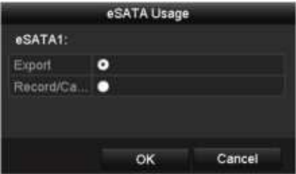
Figure 13. 22 Setting eSATA Usage
