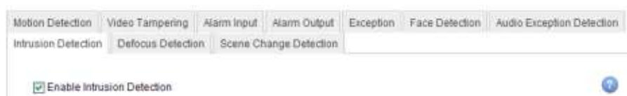
Figure 6.11 Setting Intrusion Detection on IP Camera
