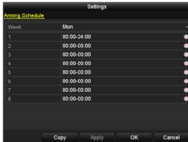
Figure 8. 17 Set Arming Schedule of Alarm Output
