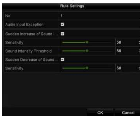
Figure 9. 9 Set Audio Exception Detection Rules
