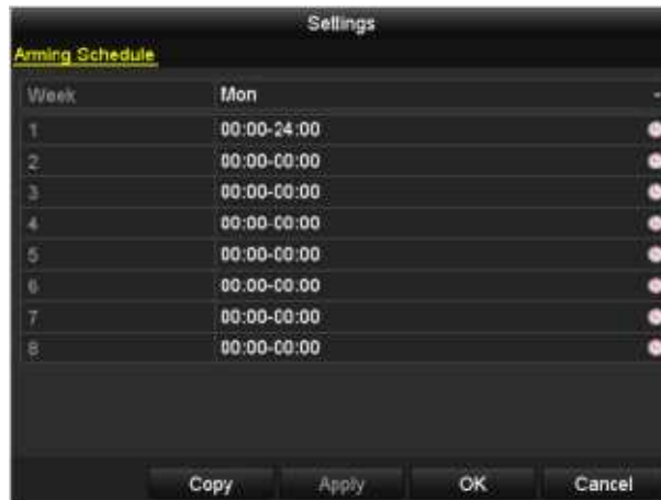
Figure 8. 17 Set Arming Schedule of Alarm Output
