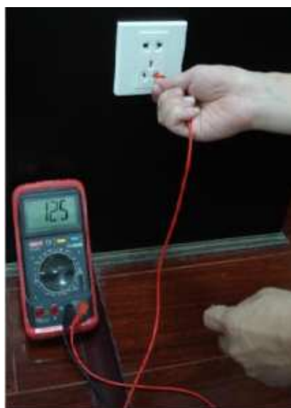
Appendix Figure 7-6 Check live cable connection
