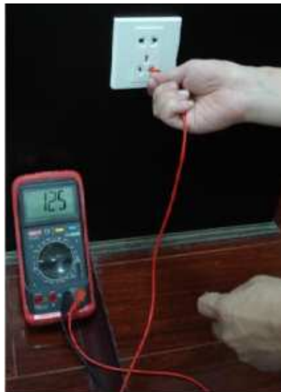
Appendix Figure 7-6 Check live cable connection
