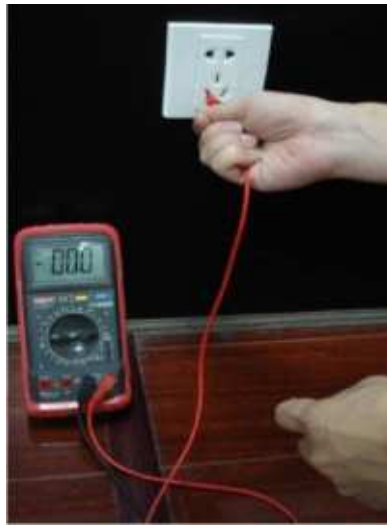
Appendix Figure 7-7 Check neutral cable connection
