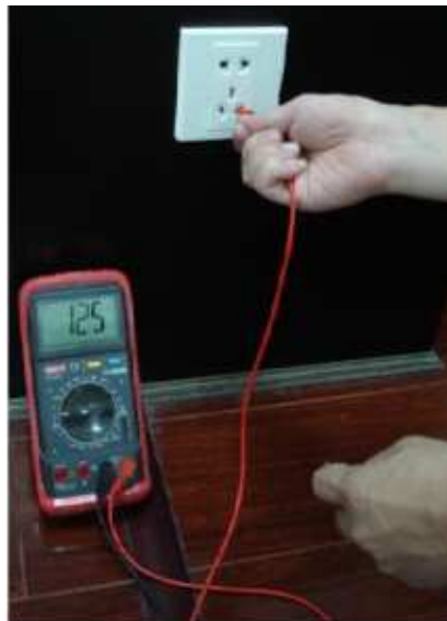
Appendix Figure 7-6 Check live cable connection
