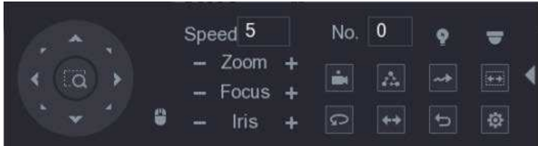
Figure 5-63 Expanded PTZ control panel
