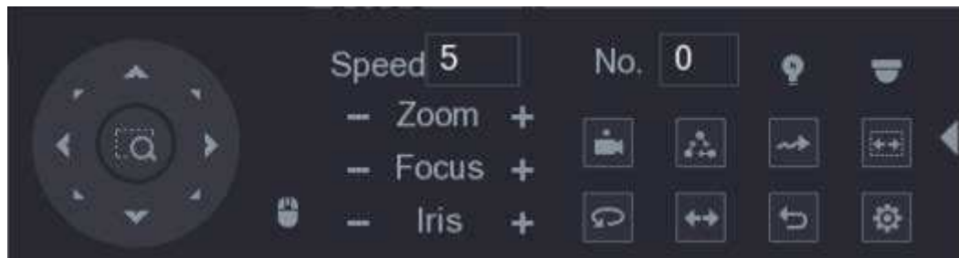
Figure 5-69 Expanded PTZ control panel
