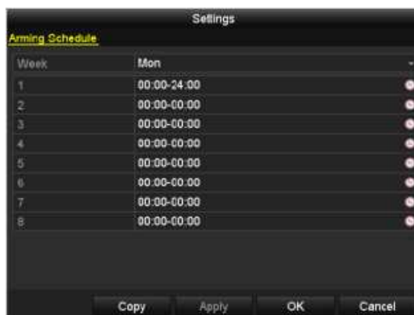
Figure 8-20 Set Arming Schedule of Alarm Output
