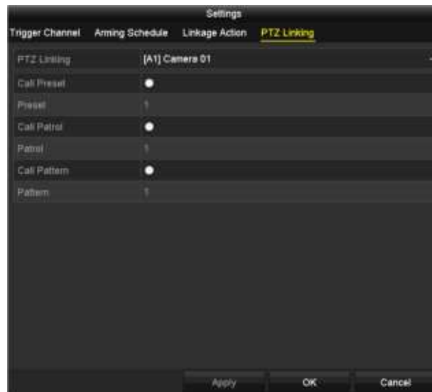
Figure 8-7 Set PTZ Linking of Alarm Input
