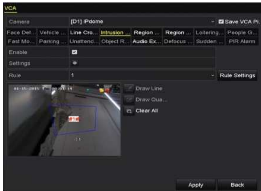
Figure 9-9 Draw Area for Intrusion Detection
