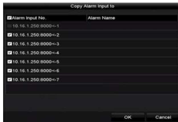
Figure 5-19 Copy Alarm Input
