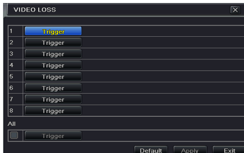
Fig 4-21 Alarm Configuration-Video Loss
