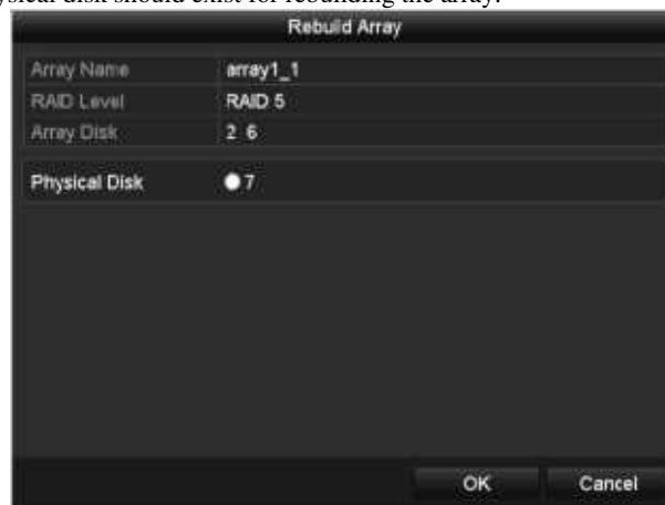
Figure 13.14 Rebuild Array Interface
