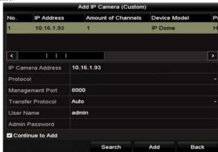
Figure 2. 26 Custom Adding IP Camera Interface
