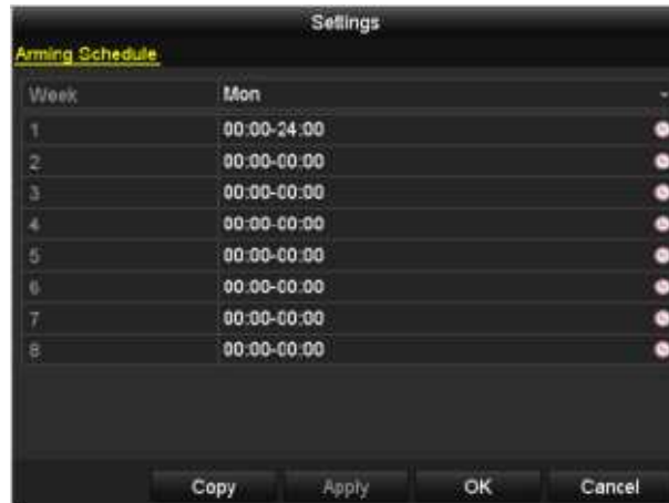
Figure 8. 20 Set Arming Schedule of Alarm Output
