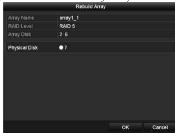
Figure 13.14 Rebuild Array Interface
