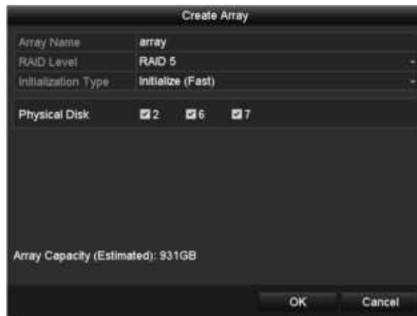
Figure 13. 8 Create Array Interface
