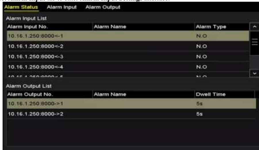
Figure 8.5 Alarm Status Interface of System Configuration
