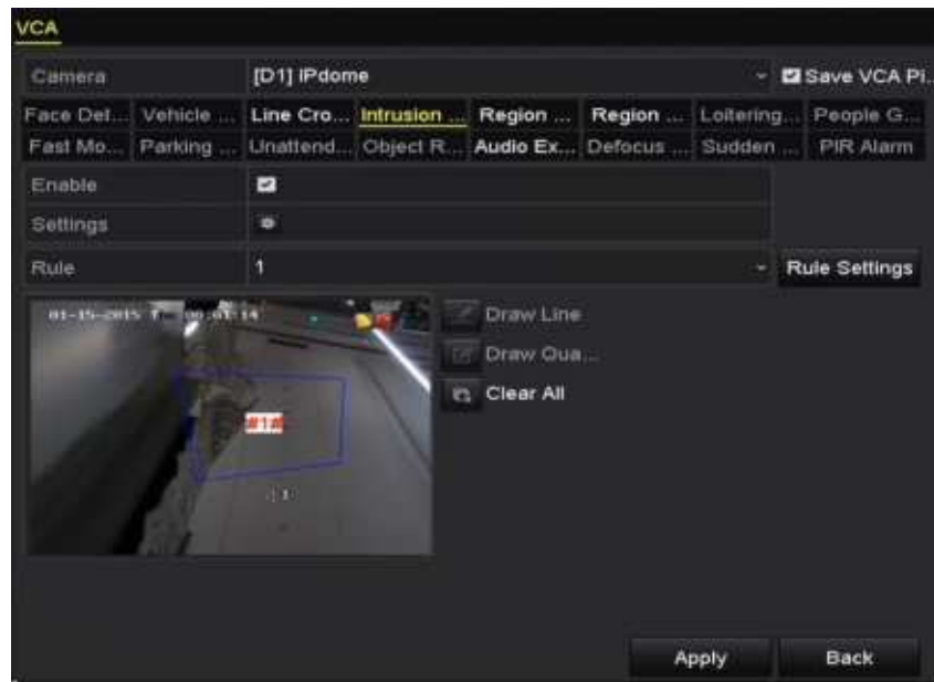
Figure 9. 6 Draw Area for Intrusion Detection
