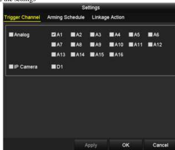
Figure 5. 19 Set Trigger Camera of VCA Alarm
