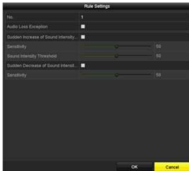
Figure 9.8 Set Audio Exception Detection Rules
