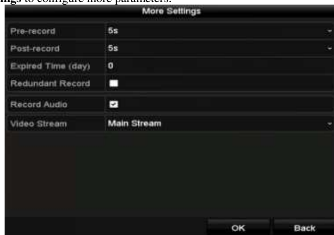
Figure 5. 4 More Settings of Record Parameters
