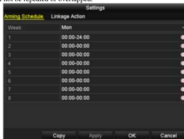
Figure 8.13 Set Arming Schedule of Video Tampering
