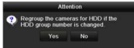
Figure 12.14 Confirm HDD Group Settings
