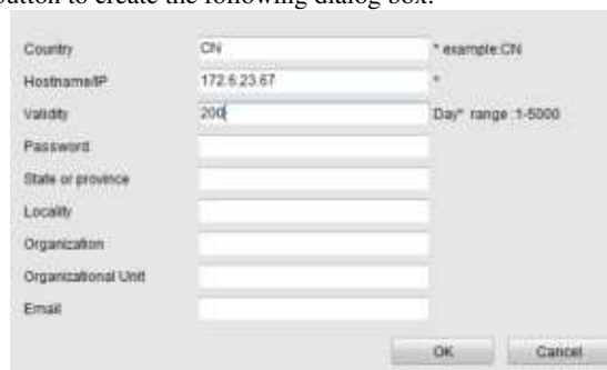
Figure 11.20 Create Self-signed Certificate
