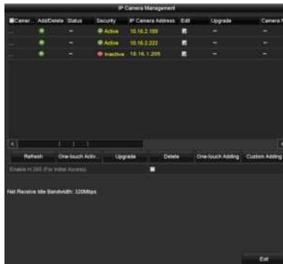
Figure 2. 21 IP Camera Management Interface
