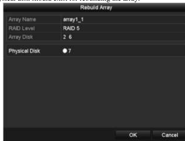
Figure 13.14 Rebuild Array Interface
