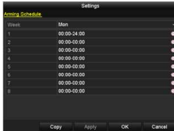
Figure 8. 20 Set Arming Schedule of Alarm Output
