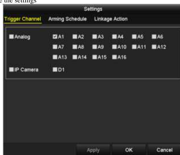
Figure 5. 20 Set Trigger Camera of VCA Alarm
