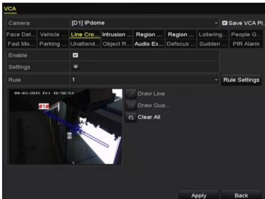
Figure 9.6 Draw Line for Line Crossing Detection
