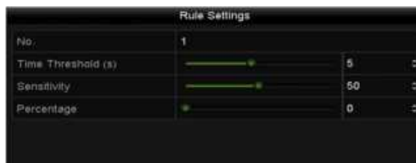
Figure 9.7 Set Intrusion Crossing Detection Rules
