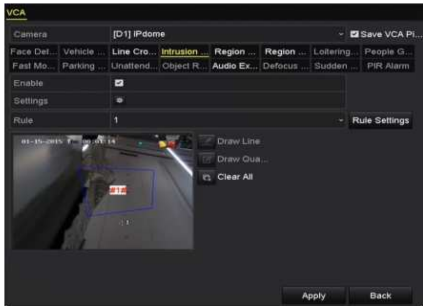
Figure 9.8 Draw Area for Intrusion Detection
