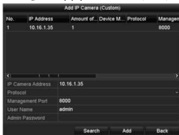
Figure 2.13 Custom Adding IP Camera Interface
