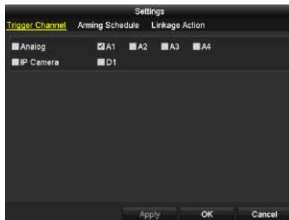
Figure 8.15 Set Triggering Channel of VCA Alarm
