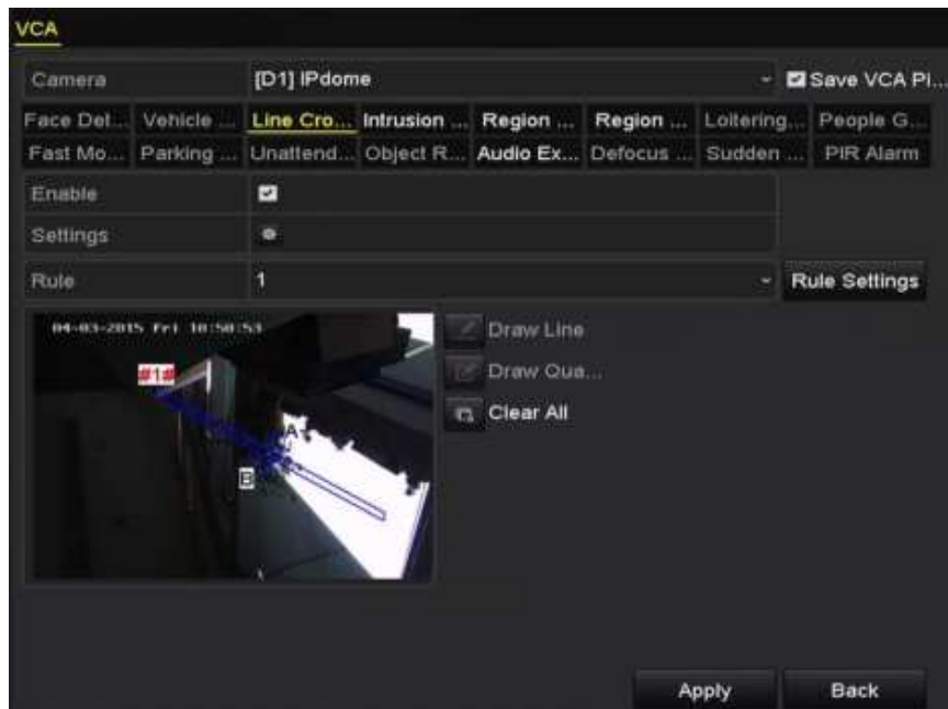
Figure 9. 4 Draw Line for Line Crossing Detection
