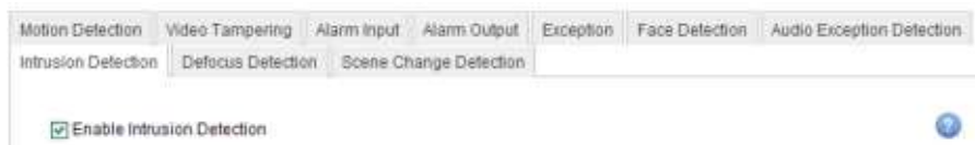
Figure 6. 13 Setting Intrusion Detection on IP Camera
