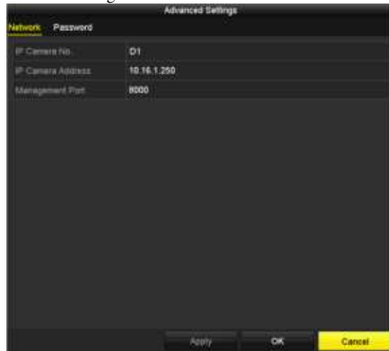
Figure 2. 28 Network Configuration of the Camera
