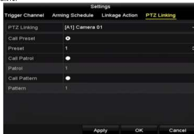
Figure 8.8 Set PTZ Linking of Alarm Input
