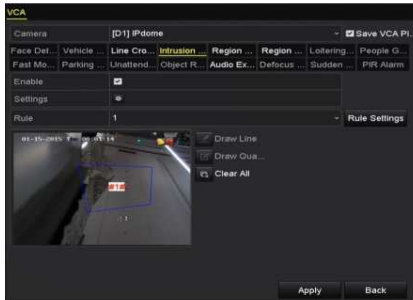
Figure 9. 6 Draw Area for Intrusion Detection
